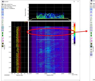
ZoomOut<sup>™</sup> display of 700 ms portion of recording. Can easily filter on both time and frequency range.
